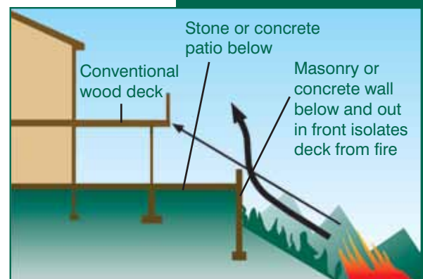
Figure 4-13: Deck with a patio and a wall below
