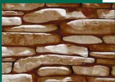
Figure 5-8: Concrete synthetic stone
